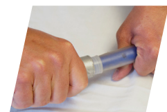
Fixing the valve and ferrule using K Crimp tube
