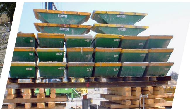
Stress test on pressure Without re-injection max. 1 500 kN With K re-injection max. 3 000 kN
