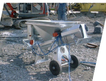
K MUNG injection system max. 70 bar injection pressure
