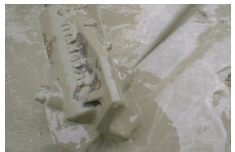
Jetting 400 bar/ KSB Jet
